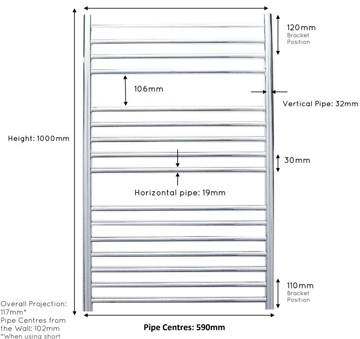
117mm\* Pipe Centres from the Wall: 102mm \*When using short brackets, projection and pipe centres from wall will be reduced by 25mm.
